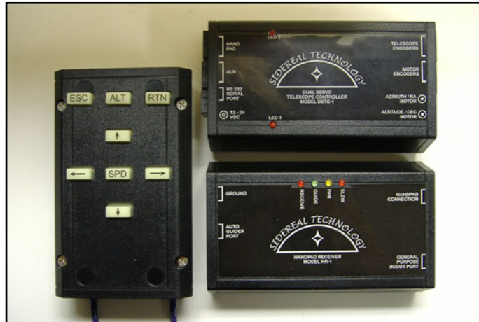
The Sidereal Technology control system handles four servo loops: typically alt and az (or RA and Dec), rotation, and focus. The ASCOM-compliant system can either operate stand-alone via a wireless (RF) control paddle, or under the supervision of a PC with control software such as Maxim DL or The Sky. Over 100 systems are in operation on a wide range of telescopes, and an active Yahoo group discusses its fine points daily.
